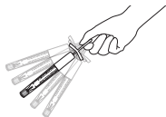
Image 2: Resetting the temperature value of the thermometer
